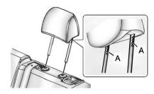
Insert the head restraint posts into the holes in the top of the seatback. The notches (A) on the posts must face the driver side of the vehicle.
