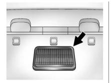
The eAssist system high voltage battery is cooled with air drawn from the vehicle interior. The cold air intake for the battery is located behind the rear seat, on the filler panel. Do not cover the intake.
