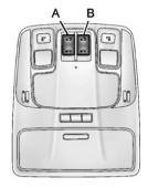
**Open/Close:** Press and hold the front or rear of switch (A) to open or close the sunroof. The sunshade automatically opens with the sunroof, but must be closed manually.
