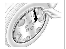
Take off the wheel cover or center cap, if the vehicle has one, to reach the wheel bolts.
