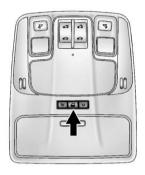
The interior lamps control located in the overhead console controls both the front and rear interior lamps.
