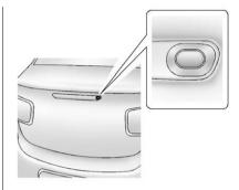
Unlock the trunk first by pressing and on the instrument panel, front door panel, or RKE transmitter. Then, press the touch pad on the trunk center high mounted stoplamp.
