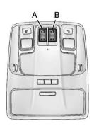
**Open/Close:** Press and hold the front or rear of switch (A) to open or close the sunroof. The sunshade automatically opens with the sunroof, but must be closed manually.
