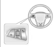
ਨ: Press to turn the cruise control system on and off. An indicator light will turn on or off in the instrument cluster.
