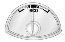
For vehicles with eAssist, this gauge assists the driver in operating the vehicle more efficiently and will vary based on driver input.
