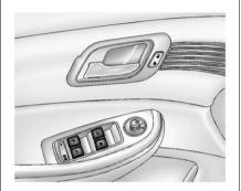
Push the switch down to open the window. Pull the front of the switch up to close it.
