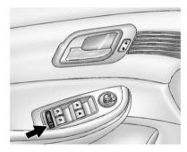
This feature prevents the rear passenger windows from operating, except from the driver position. Activating this feature will also activate the safety locks for the rear doors. See *Safety Locks on page 2-9*.
