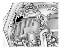
The electrical cord is located on the passenger side of the engine compartment, between the fender and the air cleaner.
