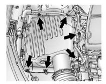
Remove the six screws on top of the engine air cleaner/filter housing.
