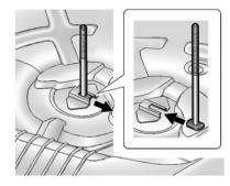
Slide the shorter bolt to remove it from the floor and insert the longer one.
