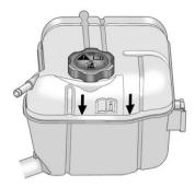
Fill the coolant surge tank with the proper mixture to the mark pointed to on the front of the coolant surge tank.
