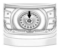
Turn the retainer nut counterclockwise and remove the spare tire. Place the spare tire next to the tire being changed.
