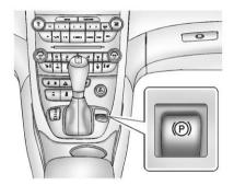
The vehicle has an Electric Parking Brake (EPB). The switch for the EPB is in the center console. The EPB can always be activated, even if the ignition is off. To prevent draining the battery, avoid repeated cycles of the EPB system when the engine is not running.
