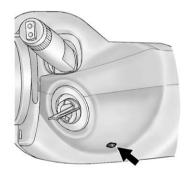
Vehicles with an automatic transmission are equipped with an electronic key lock release system. This system is to prevent ignition key removal unless the shift lever is in P (Park).
