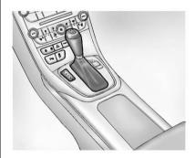
The automatic transmission has a shift lever located on the console between the seats
