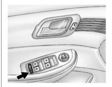
The rear door safety locks prevent passengers from opening the rear doors from inside the vehicle. Activating this feature will also activate the rear window lockout. See *Power Windows on page 2-16*.
