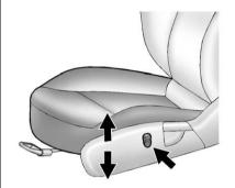
Press and hold the top or bottom of the switch to raise or lower the seat. Release the switch when the desired height is reached.
