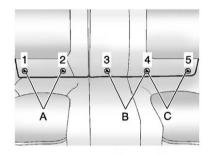
A. Passenger Side Rear Seating Position and Lower Anchors 1 and 2
