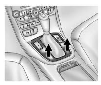
Release the shift lever trim from the center console at the rear, then fold upward and turn it to the left.
