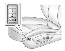
On vehicles with the memory feature, the "1" and "2" buttons on the outboard side of the driver seat are used to manually save and recall the positions of the driver seat and outside mirrors. These manually stored positions are referred to as Button Memory positions.
