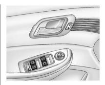
Push the switch down to open the window. Pull the front of the switch up to close it.
