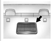
The cold air intake for the battery is located behind the rear seat, on the filler panel. Do not cover the intake. See *Battery on page 10-21*.
