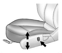
Press and hold the top or bottom of the switch to raise or lower the seat. Release the switch when the desired height is reached.
