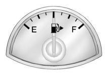
When the ignition is on, the fuel gauge shows how much fuel is left in the fuel tank. When the indicator nears empty, a message in the Driver Information Center (DIC) displays. See *Fuel System Messages on page 5-29*. The vehicle still has a little fuel left, but the vehicle should be fueled soon.
