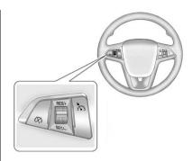
ৈ (On/Off): Press to turn the cruise control system on and off. An indicator light will turn on or off in the instrument cluster.
