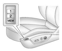
On vehicles with the memory feature, the "1" and "2" buttons on the outboard side of the driver seat are used to manually save and recall the positions of the driver seat and outside mirrors. These manually stored positions are referred to as Button Memory positions.
