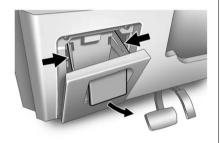
The instrument panel fuse block is located in the instrument panel, on the driver side of the vehicle. To access the fuses, open the fuse panel door by pulling down at the top.
