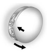
The fuel cap is behind the fuel door on the vehicle's passenger side. To open the fuel door, push the rearward center edge in and release and it will open.
