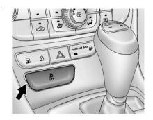
To turn the system off, press the TCS/StabiliTrak button located on the center console.
