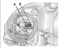
Disconnect the electrical connector (A).
