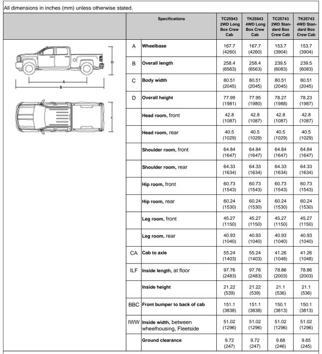
Published dimensions indicated are without optional equipment or accessories. Additional accessories or equipment ordered at the customer's request can result in a minor change in these dimensions.
