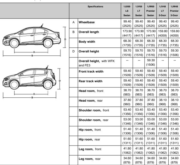
Published dimensions indicated are without optional equipment or accessories. Additional accessories or equipment ordered at the customer's request can result in a minor change in these dimensions.
